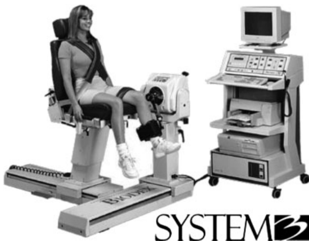
Figure 6. Biodex dynamometer for computer-controlled muscle testing (Biodex Medical Systems, Shirley, NY).
