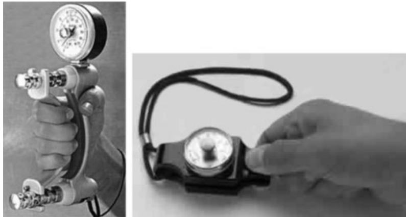
Figure 5. The Jamar hand dynamometer is pictured on the left (NexGen Ergonomics, Quebec, Canada), and the B & L Pinch Gauge is shown on the right (B & L Engineering, Tustin, CA).
