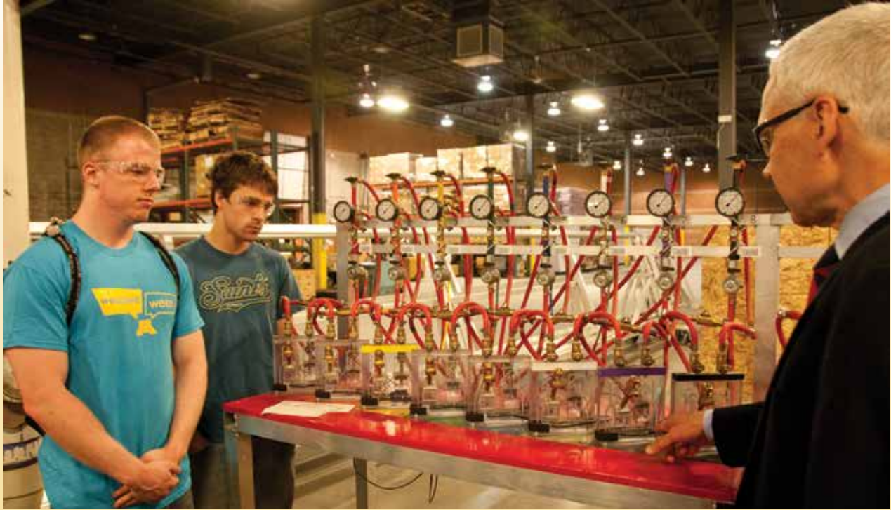
The sensing elements of the massive "bubble bottle" used to ensure that every NOvA module is free of minute leaks. If a leak exists, bubbles form in a shallow pool of water in each chamber that are "counted" by a photodetector. The basic operating principles are the same as those of a cruder device used to test for leaks in 1920's vintage player pianos.
