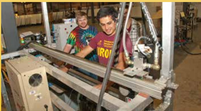
A student worker loads a NOvA module manifold cover into a glue dispensing robot. It treats the plastic surface with a corona arc to improve adhesion, then it applies a uniform bead of epoxy adhesive.
