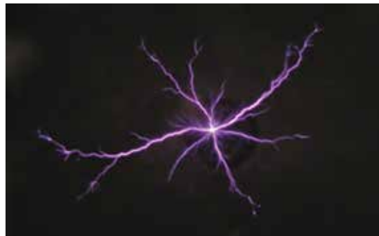
Example of a pulsed plasma produced in water. The length of the plasma filaments is about 3 cm.
