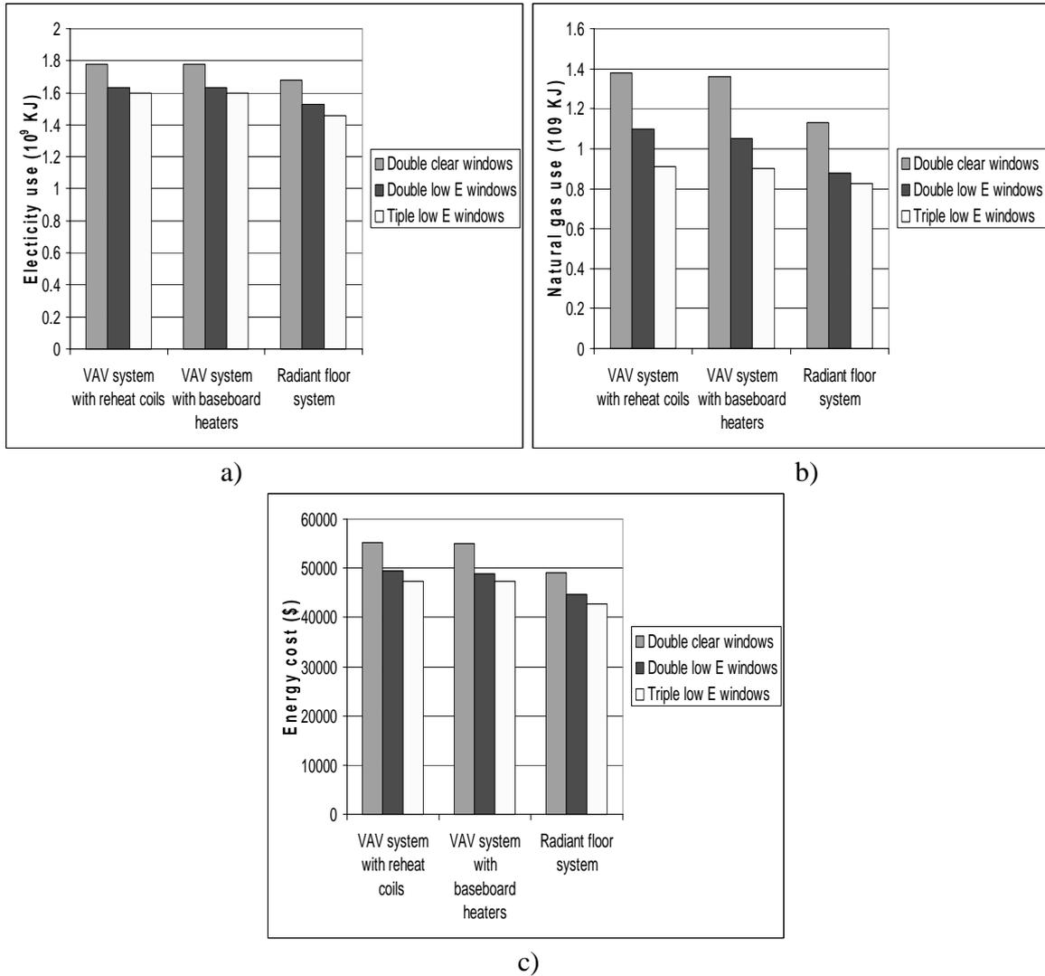
Figure 2. System comparisons. a) Annual electricity use, b) Annual natural gas use, c) Energy cost.
