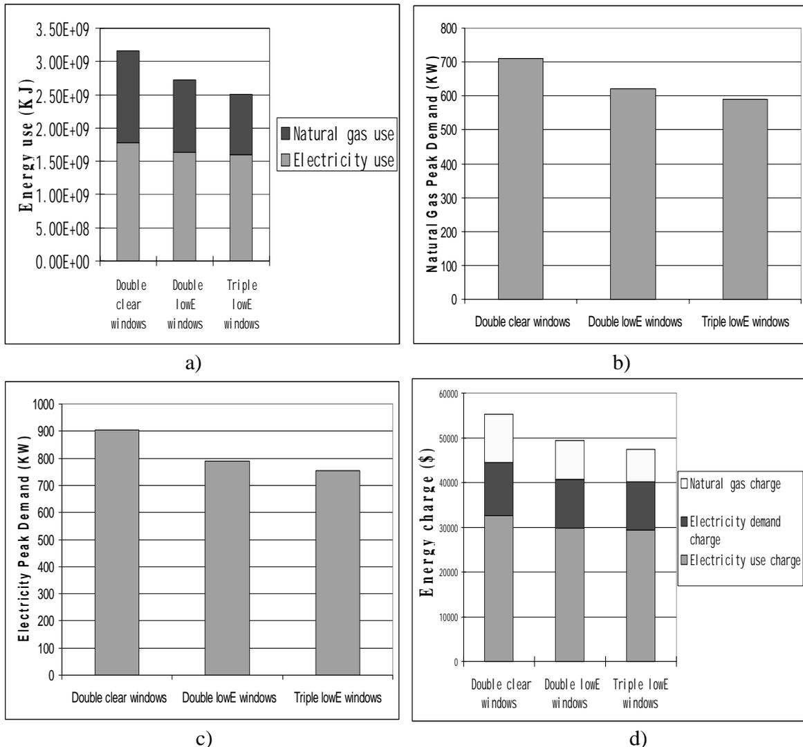
Figure 1. Comparison of energy use for a VAV system with reheat and three types of windows. a) Annual energy use, b) Natural gas peak demand, c) Electricity peak demand, d) Energy charge.
