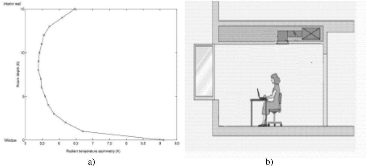
Figure 3. a) Radiant temperature asymmetry for the perimeter room with double low E windows, b) Perimeter zone with VAV system.
