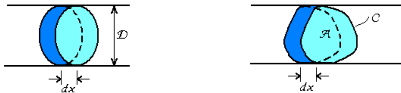
Fig. 9.3 Control volumes for the analysis of fully developed flow in circular pipes and non-circular ducts
