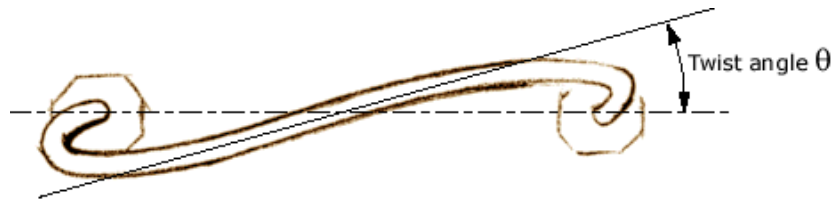
A snapshot of flow tube inside Coriolis flowmeter
